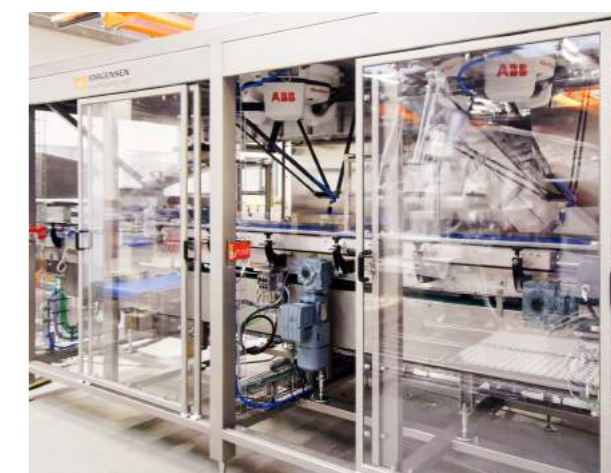
Complete pick & place system with 2 robots
