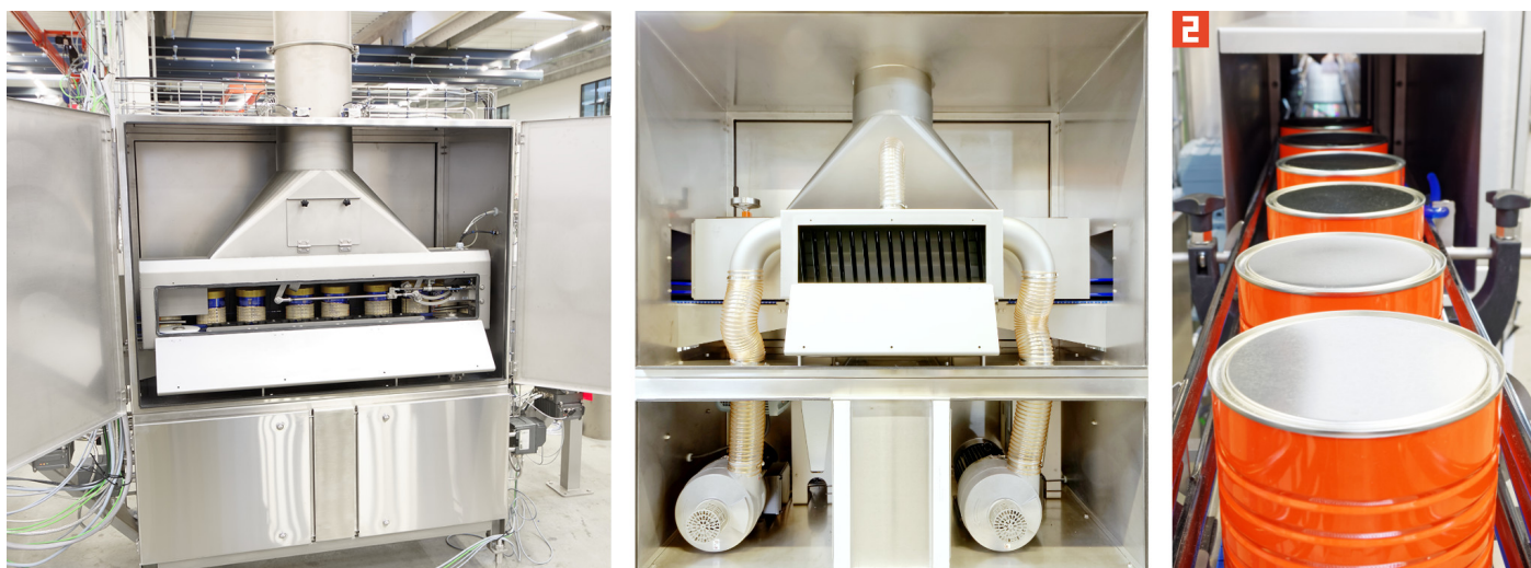
1: Can cleaner and dust extraction system. 2: Clean can surfaces after cleaning procedure.
