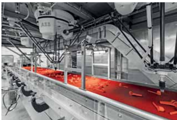
Robotic milk powder handling: efficient, flexible and reliable scoop inserting.
